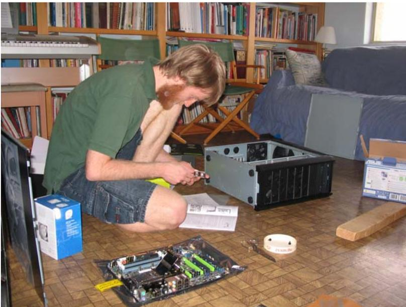
Get out the motherboard. Place the motherboard I/O shield into the slot in the case.
