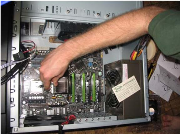
Place the CPU in the CPU socket on the motherboard. Apply thermal paste to CPU.
