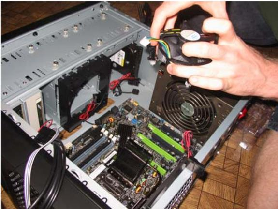
Attach the CPU heat sink.
